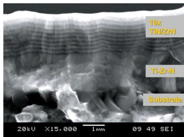
Fig. 2. Example of structure of multilayer PVD coating of Ti-Zr-N/10x(TiN/ZrN) type developed in IAMT, deposited on the cutting edge - electron micrograph.
