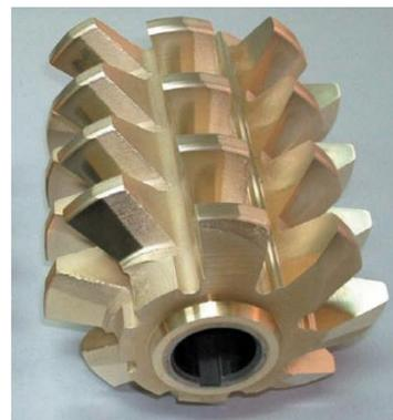
Fig. 5. High-speed steel gear cutting hob with module  $m = 10$  mm with multilayer coating 11x(TiN/ZrN) deposited by PVD arc-plasma method in IAMT
