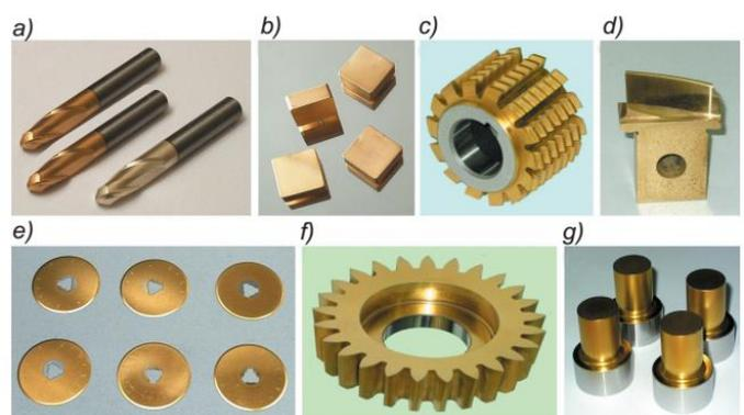
Fig. 6. Examples of tools with multilayered coatings deposited in IAMT: a) ball nose endmills, b) cutting inserts, c) gear cutting hob, d) blade for Gleason cutter head, e) circular cutting knives, f) Fellows gear shaper cutter, g) punches
