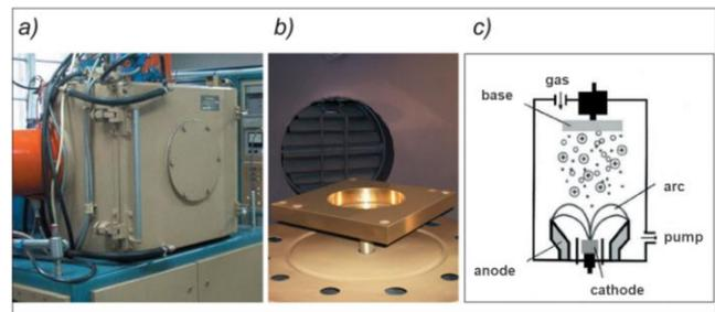
Fig. 1. View of the chamber (a) of the PVD arc-plasma device owned by IAMT; inside the chamber - a part with deposited coating (b) and the principle of the device operation (c)
