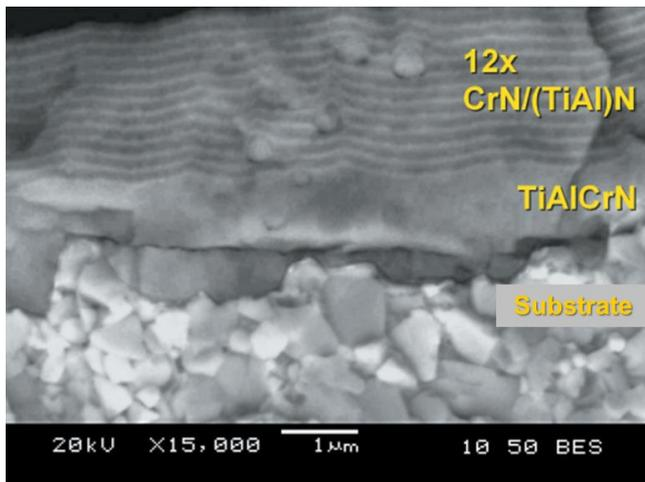
Fig. 4. Example of structure of multilayer PVD coating of TiAlCrN/12x(CrN/(TiAl)N) type developed in IAMT, deposited on the cutting edge - electron micrograph.
