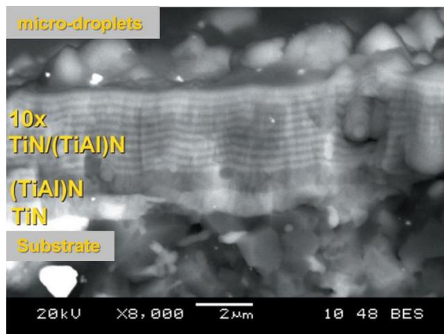
Fig. 3. Example of structure of multilayer PVD coating of TiN/(TiAl)N/10x(TiN/(TiAl)N) type developed in IAMT deposited on the cutting edge - electron micrograph.
